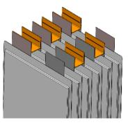
Laser lap joint for punch
