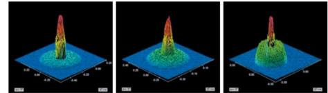
Flexible setting of the intensity distribution with BrightLine Weld.
