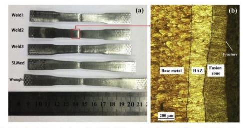
Fig. 11. Photos of tensile test samples after tensile tests (a) and OM image showing fracture path of laser-welded joint under type 2 (b).
