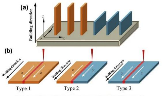
Fig. 2. Schematic drawings of SLMed plates (a) and different laser welding types (b).
