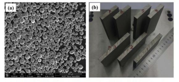
Fig. 1. Morphology of metal powders (a) and macro-morphology of SLMed plates (b) of 304 stainless steel.
