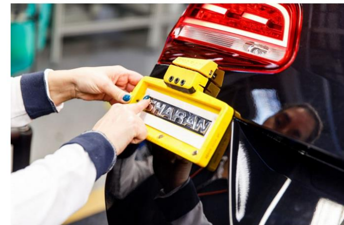
A 3D printed liftgate badge tool, used to accurately apply a car's model name. Photo via Ultimaker
