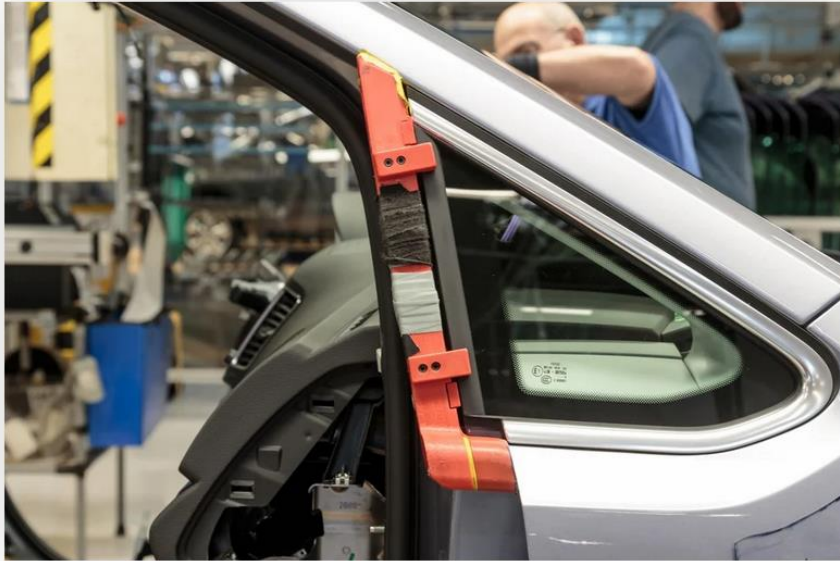
A 3D printed jig on a Volkswagen assembly line. (Source: Volkswagen)
