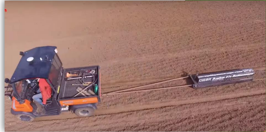
EC/EM mittausta, Dualem 21s soilscanner
